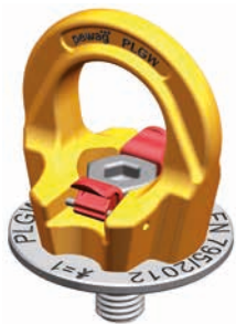
Image 3: Position ‚A‘ – both latches are touching the screw. Only permitted during mounting and demounting.
