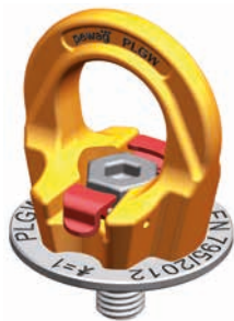
Image 4: Position ‚B‘ – none of the latches is touching the screw. The anchoring point is only ready to be used in this position.
