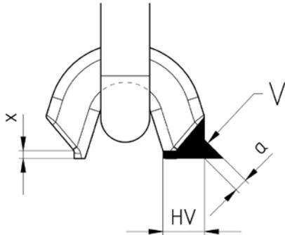
Picture 2: Weld seam geometry
