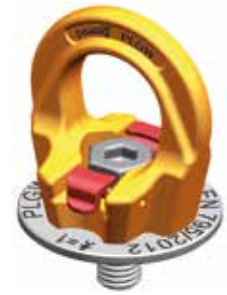
Image 4: Position ,B' – none of the latches is touching the screw. The anchoring point is only ready to be used in this position.
