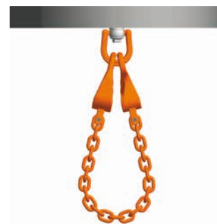
Fig. 6: Correct assembly of the sleeve
