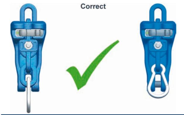
Figure 10 – Correct assembly of the stopper set
