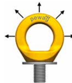
Fig. 1: Permitted directions of load that occur during correct use.
