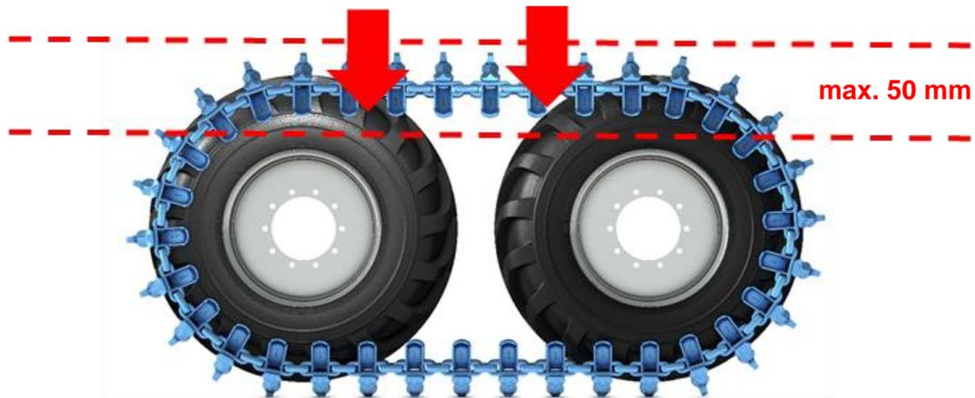
A certain level of usage-induced wear is normal for pewag bluetracks and will cause them to rest on the tyre more loosely. This means that they may lose some tension and slip off the tyre, which is why systematic re-tensioning is so important. In the following steps, we will show you how to do this correctly.
